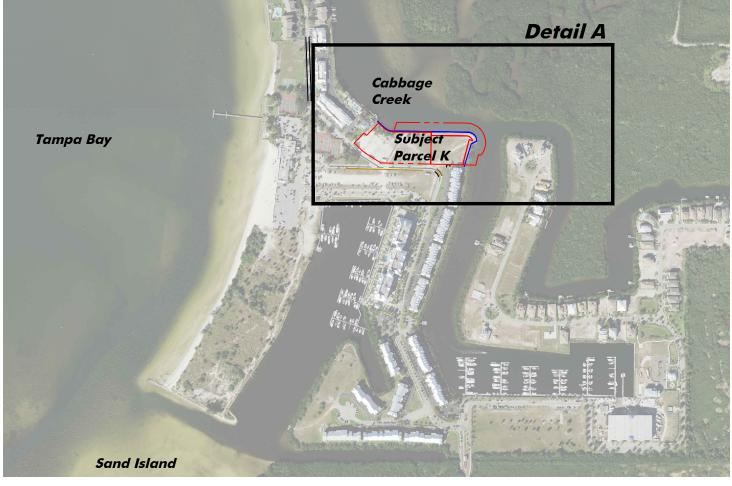
Note: Field work completed 6-9-2023 by Hans Wilson and Associates, Inc. All topographic elevations reference NAVD88. Bathymetric survey references Tide Station 872-6384. MHW @ 0.32' NAVD and MLW @ -1.23' NAVD.
